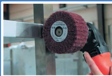
Finish of square constructions
